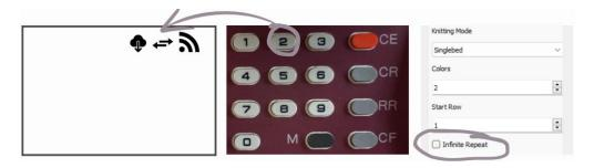
Without Download Feature on: Activate the infinite repeat directly in the eKnitter-AYAB software to allow the pattern to continuously repeat.
