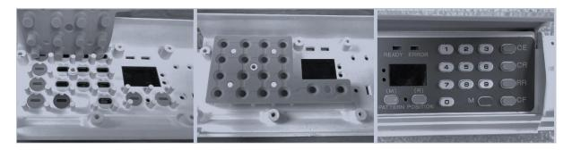
**Position the eKnitter Board:** Place the eKnitter board in its designated spot, aligning the board's screw holes directly above the corresponding screw holes on the lid.
